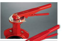
**PADLOCK KIT** allows the customer to lock the valve in the full open or closed position, tamper proofing the valve. By drilling a new hole in the top plate, the handle can be locked in mid travel.
