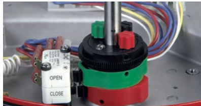
INFINITELY ADJUSTABLE TRAVEL LIMIT CAMS
