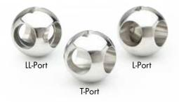
Multi-Port ball valves offer a wide range of flow patterns: 90° and 180° T & L port 3-way balls, and 90°, 180° and 270° 4-way balls. Features include a 4th seat to prevent leakage and maintain proper ball alignment, live loaded stem seal and locking handles.
