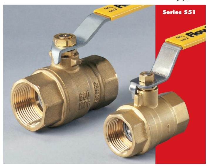
Flow-Tek's Series S51 brass ball valves are the ideal utility valve for low pressure commercial applications. The two-piece body construction offers simple quarter turn operation, low operating torque and bottom entry blowout proof stems. The balls are hard chromium plated brass for added durability and longevity. The Series S51's full port design minimizes pressure drops while maximizing flow.
