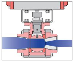
Media Flow entering valve from the left. Installing the V downstream is preferred.
