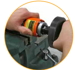
Change from OD to ID skiving tool in seconds with PTO coupling
