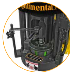
Coupling Stop makes repetitive crimps faster
