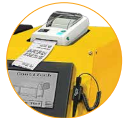
Results of each test are recorded and can be printed on the included printer or saved via USB port
