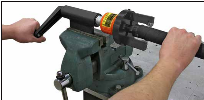
Laser etched scale is designed to help accurately calibrate the skive diameter
