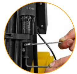
Easy calibration adjustment to increase or decrease the crimp diameter
