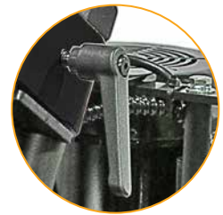
Retraction Stop limits ram retraction for quick repetitive crimps
