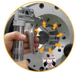
Easy grease maintenance through the 8 lubrication fittings
