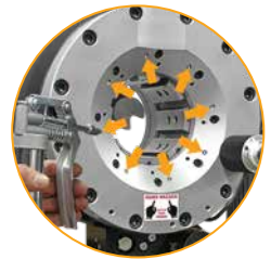
Easy grease maintenance through the 8 lubrication fittings
