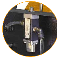
Safety Switch activates and drops pressure as soon as the lid is opened
