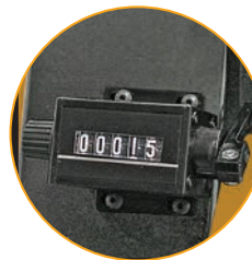
A resettable counter makes it easy to keep track of the number of cuts made
