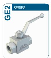
Number of Ports: 2 Material: Available in carbon steel and stainless steel Available Sizes: ¼ to 1" Port: NPT, BSP, SAE, Flange Operating Pressure: Up to 500 bar Temperature range: -60 + 230 °C (dependent on body and seal material)
