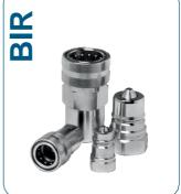
Valving Style: Poppet Interchange: ISO 7241 'A' Sealing description: Nitrile NBR Available sizes: From 1/4" to 2" Operating Pressure: Up to 350 bar Flow rate: Up to 1000 L/min Material / Treatment: Carbon steel / Cr3 Connection under pressure: Allowed (only PC version)
