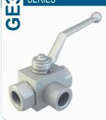
Number of Ports: 3 Port Type: L and T Material: Available in carbon steel and stainless Available Sizes: ¼ to 1" Port: NPT, BSP Operating Pressure: Up to 400 bar Temperature range: -60 + 230 °C (dependent on body and seal material)
