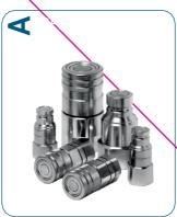
Valving Style: Flat face Interchange: ISO 16028 Sealing description: Nitrile NBR Availablesizes: From 1/8" to 1-1/2" Operating Pressure: Up to 420 bar Flow rate: Up to 750 L/min Material/treatment: Carbon steel/Cr3
