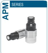
Interchange: ISO 16028 and NFPAT3.20.15 HTMA (size 3/8") Available Sizes: From 3/8" to 1-1/2" Operating Pressure: Up to 350 bar Flow rate: Up to 750 L/Min Material/treatment: Carbon steel/Cr3 Connection system: Push Connection under pressure: Male side, other side to drain
