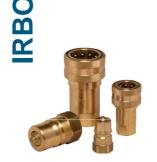
Valving Style: Poppet Interchange: ISO 7241-1 "B" Available sizes: From 1/8" to 1" Operating Pressure: Up to 200 bar Flow rate: Up to 200 L/Min
