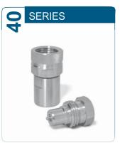
Valving style: Poppet Interchange: VVS Interchange Available sizes: From 1/4" to 2" Operating pressure: Up to 650 bar Flow rate: Up to 750 L/Min Material: 316L
