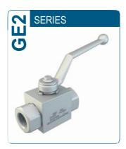
Number of Ports: 2 Material: Available in carbon steel and stainless steel Available Sizes: 1/4 to 1" Port: NPT, BSP, SAE, Flange Operating Pressure: Up to 500 bar Temperature range: -60 + 230 °C (dependent on body and seal material)
