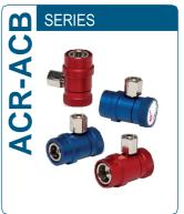
Valving style: Poppet Interchange: SAE J639 Sealing description: HNBR Available Sizes: 1/4" Operating Pressure: Up to 10 bar Flow rate: Up to 750 l/min Material / Treatment: Brass
