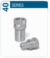
Valving style: Poppet Interchange: VVS Interchange Available Sizes: From 1/4" to 2" Operating Pressure: **Up to 650 bar** Flow rate: Up to 750 L/min Material: 316L Connection system: Screw Connection under pressure: One side
