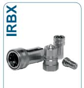
Valving style: Poppet Interchange: ISO 7241 'B' Sealing description: FKM (Viton®) Available sizes: From 1/8" to 1" Operating pressure: Up to 250 bar Flow rate: **Up to 200 I/min**Material / Treatment: **316L**
