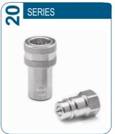
Valving style: Poppet Interchange: ISO 7241-1 A Available sizes: From 1/4" to 2" Operating pressure: **Up to 350 bar** Flow rate: **Up to 1000 L/Min** Material: 316L Connection system: Single acting sleeve Connection under pressure: Not allowed
