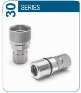
Valving style: Poppet Interchange: ISO 14541 Available sizes: From 1/4" to 1 1/4" Operating pressure: Up to 450 bar Flow rate: Up to 378 L/Min Material: 316L Connection system: Screw
