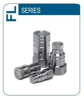
Valving style: Flat face Interchange: ISO 16028 Sealing description: FKM (Viton®) Available sizes: From 1/8" to 2" Operating pressure: Up to 350 bar Flow rate: Up to 1000 I/min Material / Treatment: 316L
