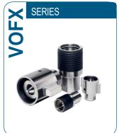
Valving style: Poppet Interchange: With similar couplings Sealing description: Nitrile NBR Available sizes: From 3/4" to 2" Operating pressure: Up to 207 bar Flow rate: Up to 1100 l/min Material / Treatment: 316L Connection under pressure: Allowed
