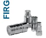
Valving Style: Flat face Interchange: ISO 16028 and NFPA T3.20.15 HTMA (size 3/8") Available sizes: From 1/8" to 1-1/2" Configuration: Modular construction Operating Pressure: Up to 420 bar Flow rate: Up to 750 L/Min Material / Treatment: Carbon steel/ Cr3 (Zi-Ni version available) Connection system: Push Connection under pressure: Not allowed
