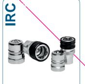
Valving Style: Poppet Interchange: similar couplings (Nordic interface) Available sizes: From 1/4" to 1" Operating Pressure: Up to 600 bar Flow rate: Up to 378 L/min Material / Treatment: Carbon steel / Cr3 Connection system: Single acting sleeve Connection under pressure: One side with PC version
