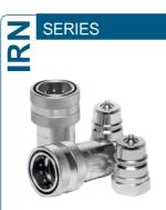
Valving style: Poppet Interchange: Similar Couplings Available sizes: 1" Operating Pressure: Up to 300 bar Flow rate: Up to 378 L/min Material / Treatment: High strength carbon steel Connection system: Single active sleeve Connection under pressure: Not allowed
