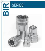
Valving style: Poppet Interchange: ISO 7241-1 "A" Available Sizes: From 1/4" to 2" Operating Pressure: Up to 350 bar Flow rate: Up to 1000 L/min Material: Carbon steel/Cr3 Connection system: Single acting sleeve Connection under pressure:: One side with PC version
